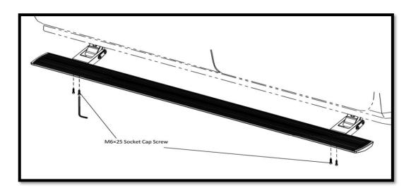
**Step 5**: Install the Passenger side running board. With assistance, begin by positioning the board on the front and rear motor assembly bases. Align the sliding T-Nut on the running board with the slots on the front and rear motor base. Once the T-Nuts are aligned, rotate the running board so that the T-Nuts set in the slots on the base of the arms. Repeat Steps 2-9 to install the motor linkage assemblies and running board on the Driver side.
