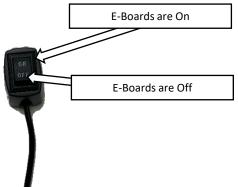
**Step 21:** Open the Driver side door and keep the door open. Flip the disable switch to the Off position. This will signal the running boards to retract to the stowed position and it will disable any further operation until the switch is flipped to the On position.
