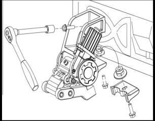
**Step 3:** Install front Passenger and rear Passenger side motor using M8x30 Hex Flange Bolt on the top mounting hole and M8x25 on the bottom mounting hole. Use M8 Flat washer and M8 Hex nut on the bottom mounting hole.
