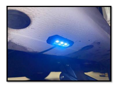
**Step 10**: Align the arrows on the small round connectors and plug the Passenger side front and Passenger side rear LED lights. Prepare the surface by cleaning with a 50/50 mix of isopropyl alcohol and water or equivalent. Once the surface is completely dry, peel the backing from the double-sided tape and stick the LEDs to the bottom side of the rocker panel. Position the LED lights at the center of the front and rear passenger side doors
