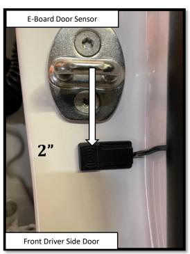
**Step 14: FRONT DOOR** Apply a vertically oriented strip of masking tape on the front passenger side door using the deepest part of the latch as a reference point. Make a mark 2" below the center line of the latch. Prepare the surface by cleaning with a 50/50 mix of isopropyl alcohol and water or equivalent. Once the surface is completely dry, peel the backing from the double-sided tape and stick the magnet to the door. Align the top of the magnet with the 2" mark as shown.
