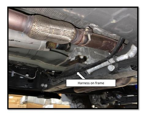
**Step 11**: Route the motor and LED wire harness from the controller to the Driver side frame rail of the vehicle. When routing the harness keep clear from any moving parts and avoid direct contact with the exhaust system.
