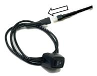
**Step 19:** Locate the black wires for the disable switch and feed them to your desired mount location. Prepare the surface by cleaning with a 50/50 mix of isopropyl alcohol and water or equivalent. Once the surface is dry, peel the backing from the double-sided tape and stick the disable switch on the lower dash panel. Plug the disable switch connector into the black wire harness and tuck the extra wire behind the lower dash panel.
