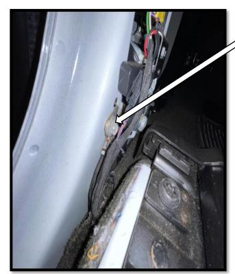
**Step 19:** The door trigger sensor harness will need a ground connection to the vehicle. Locate the seat belt assembly at the passenger side b-pillar and install the ground wire under the top bolt of the seat belt assembly.
