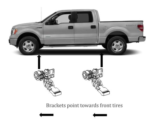
**Step 9**: Repeat Steps 1-8 to install the motor bracket assemblies and running board on the driver side.
