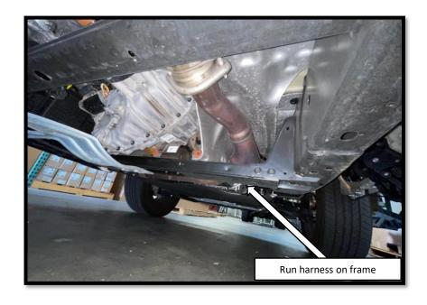
**Step 12**: Route the motor and LED wire harness from the controller to the DRIVER side frame rail of the vehicle. When routing the harness keep clear from any moving parts and avoid direct contact with the exhaust system.
