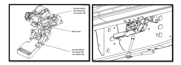
**Step 5**: Fasten the bottom of each motor with two (2) M8x30 Hex Bolts, two (2) M8 Flat Washers, two (2) Lock Washers to the pinch weld
