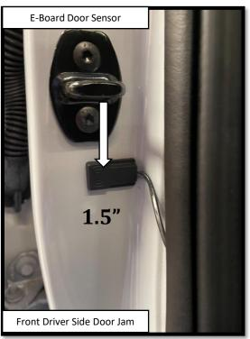
Step 17: FRONT DOOR Apply a vertically oriented strip of masking tape on the front Passenger side door using the deepest part of the latch as a reference point. Make a mark 1.5" below the center line of the latch. Prepare the surface by cleaning with a 50/50 mix of isopropyl alcohol and water or equivalent. Once the surface is completely dry, peel the backing from the double-sided tape and stick the magnet to the door. Align the top of the magnet with the 1.5" mark as shown.
