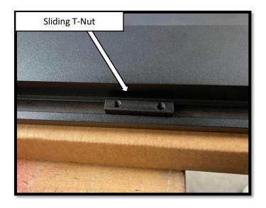
**Step 7**: Install the Passenger side running board. With assistance, begin by positioning the board on the front and rear motor assembly bases. Align the sliding T-Nut on the running board with the slots on the front and rear motor brackets. Once the T-Nuts are aligned, rotate the running board so that the T-Nuts set in the slots on the base of the arms.
