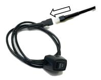
**Step 22:** Locate the black wires for the disable switch and feed them to your desired mount location. Prepare the surface by cleaning with a 50/50 mix of isopropyl alcohol and water or equivalent. Once the surface is dry, peel the backing from the double-sided tape and stick the disable switch on the lower dash panel. Plug the disable switch connector into the black wire harness and tuck the extra wire behind the lower dash panel.
