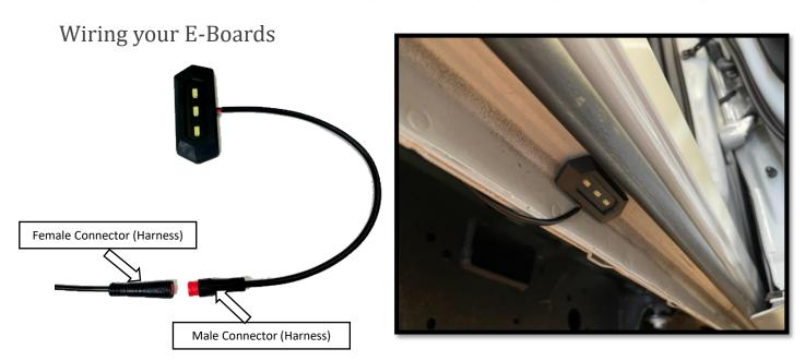
**Step 11**: Align the arrows on the small round connectors and plug the Passenger side front and Passenger side rear LED lights. Prepare the surface by cleaning with a 50/50 mix of isopropyl alcohol and water or equivalent. Once the surface is completely dry, peel the backing from the double-sided tape and stick the LEDs to the bottom side of the rocker panel. Position the LED lights at the center of the front and rear passenger side doors
