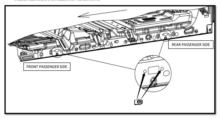
Step 3: Locate front and rear mounting provisions and install two (2) clip nuts per side
