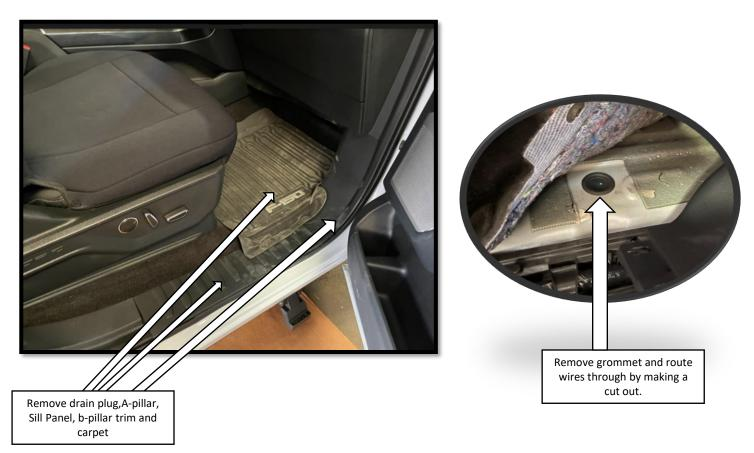
**Step 14:** Go under the vehicle and feed the door trigger signal wires (white and brown) and the disable switch wires (two black wires) into the cab. Feed the wires thru the hole in the rubber drain plug. Pop the grommet back into the slot. Seal around the wires using RTV silicone adhesive to prevent water intrusion.
