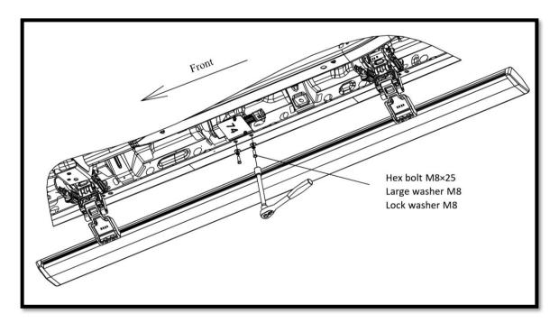
**Step 6**: Fasten the control module of each motor with two (2) M8x25 Hex Bolts, two (2) M8 Flat Washers, two (2) Lock Washers to the pinch weld on the center of the cab.
