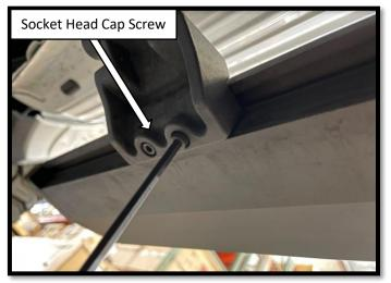
**Step 8**: Determine where you want to position the board and secure the running board to the arms using the (2 per bracket) M6x25 socket head cap screws. Using a torque wrench, tighten to 9 ftlbs. With the running board installed, fasten the hardware on the Passenger side front and rear motor assemblies. Using a torque wrench, tighten the mounting hardware to 18 ft-lbs.
