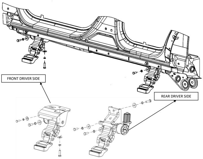
**Step 3**: Install the front driver side motor using (2) M8x25MM hex bolts, (2) M8 Lock Washer, (2) M8 Flat Washer on the pinch weld and (1) M10x35MM hex bolts, (1) M10 Lock Washer, (1) M10 Flat Washer on the rocker panel, to fasten the motor to the vehicle. The hardware should be hand tightened only until snug. This will allow the motor assembly to move and align easier when installing the running board.
