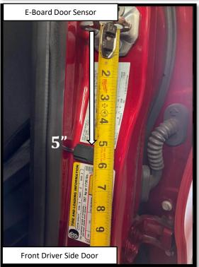
**Step 16: FRONT DOOR** Apply a vertically oriented strip of masking tape on the front driver side door using the deepest part of the latch as a reference point. Make a mark 5" below the center line of the latch. Prepare the surface by cleaning with a 50/50 mix of isopropyl alcohol and water or equivalent. Once the surface is completely dry, peel the backing from the double-sided tape and stick the magnet to the door. Align the top of the magnet with the 5" mark as shown.
