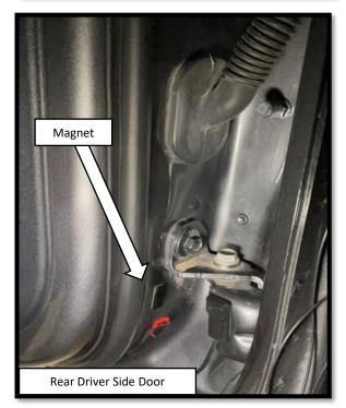
**Step 18: REAR DOOR** Prepare the surface of the bottom door hinge by cleaning with a 50/50 mix of isopropyl alcohol and water or equivalent. Lift the bulb door seal to route the sensor wire underneath it. Once the surface is completely dry, peel the backing from the double-sided tape and stick the rear door sensor to the bottom door hinge.
