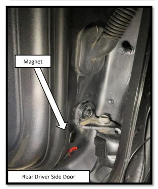
**Step 18: REAR DOOR** Prepare the surface of the bottom door hinge by cleaning with a 50/50 mix of isopropyl alcohol and water or equivalent. Lift the bulb door seal to route the sensor wire underneath it. Once the surface is completely dry, peel the backing from the double-sided tape and stick the rear door sensor to the bottom door hinge.
