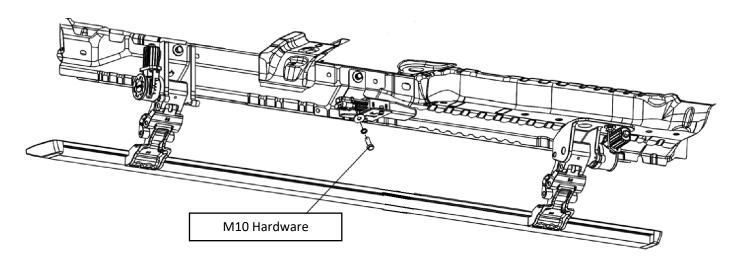
**Step 5**: Locate the threaded holes near the center of the cab on the Driver side of the vehicle. Install the controller bracket using (2) M10x25MM hex bolts M10 Lock Washer, M10 Flat Washer, to fasten the control module to the vehicle.
