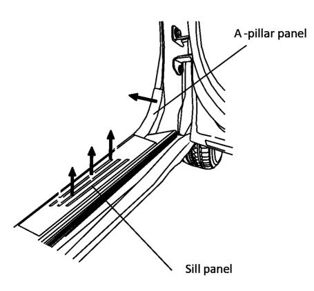
Step 14: On the Passenger side, remove the front kick panel, front door sill trim panel, and b-pillar trim panel. Pull the front passenger carpet back and cut a 7/16" hole on the rubber gromet as shown. Feed the door trigger signal wires (white and brown) and the disable switch wires (two black wires) into the cab. Seal around the wires using RTV silicone adhesive to prevent water intrusion.
