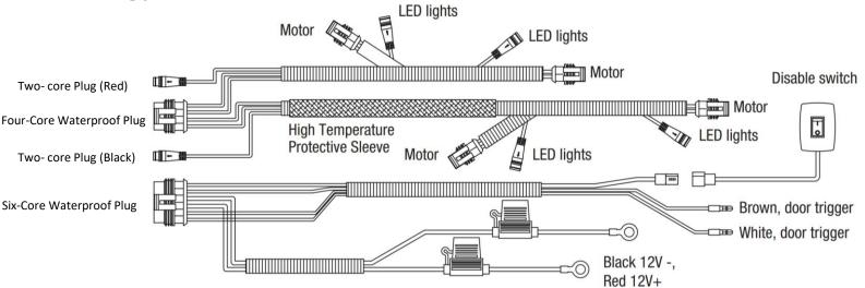
**Step 11:** Route the electrical harness from the controller along the frame rail of the truck. Connect the male plug connector on the wire harness into the female socket on the motors. The harness is labeled to show where to plug each male connector to the female connector. For example, Front Left is for the front Driver side motor and Rear Left for the rear Driver side motor. Use supplied zipties to secure harness to the frame rail.
