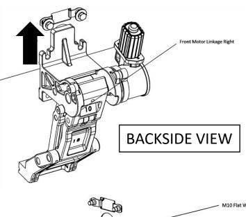
**Step 5**: Install the Front Passenger side motor using (2) hex bolts, (2) M8 Flat Washers, (2) M8 Lock Washers into the front mounting holes of the pinch weld to fasten the motor to the truck. The hardware should be hand tightened only until snug. This will allow the motor assembly to move and align easier when installing the running board.
