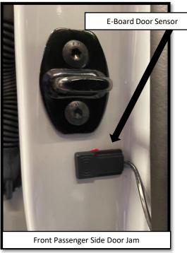
Step 17: FRONT DOOR Apply a vertically oriented strip of masking tape on the front driver side door using the deepest part of the latch as a reference point. Make a mark 2-3" below the center line of the latch. Prepare the surface by cleaning with a 50/50 mix of isopropyl alcohol and water or equivalent. Once the surface is completely dry, peel the backing from the double-sided tape and stick the magnet to the door. Align the top of the magnet with the 5" mark as shown.
