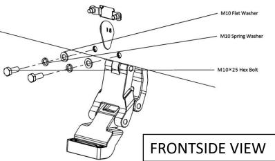
**Step 6**: Install the Rear Passenger side motor using (2)M10 hex bolts, (2) M10 Flat Washers, (2) M10 Lock Washers into the front mounting holes of the pinch weld to fasten the motor to the truck. The hardware should be hand tightened only until snug. This will allow the motor assembly to move and align easier when installing the running board.
