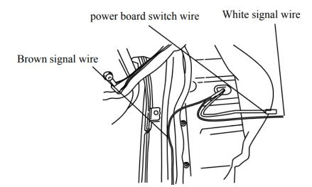
**Step 14:** Go under the vehicle and feed the door trigger signal wires (white and brown) and the disable switch wires (two black wires) into the cab. Feed the wires thru the hole in the rubber drain plug. Pop the drain plug back into the slot. Seal around the wires using RTV silicone adhesive to prevent water intrusion. These cables will run underneath the driver side seat.
