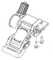
**Step 5**: Install the REAR DRIVER side motor using (2) M8X30mm Flange Bolts, to fasten the motor to the vehicle. The hardware should be hand tightened only until snug. This will allow the motor assembly to move and align easier when installing the running board.
