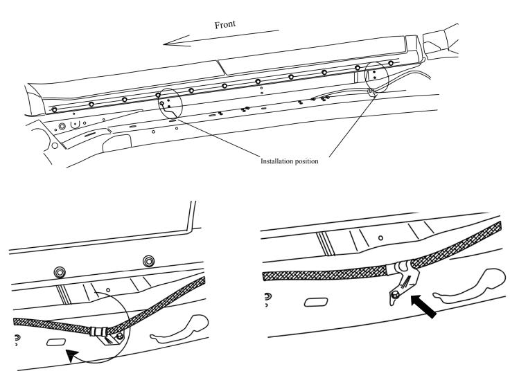
**Step 3**: On the driver side rear, locate the parking brake bracket and separate it from the wire. Rotate the bracket 180° (Located at the rear of the truck)
