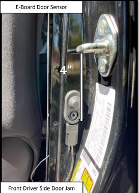
**Step 17: FRONT DOOR** Apply a vertically oriented strip of masking tape on the front Driver side door using the deepest part of the latch as a reference point. Make a mark 3.5" below the center line of the latch. Prepare the surface by cleaning with a 50/50 mix of isopropyl alcohol and water or equivalent. Once the surface is completely dry, peel the backing from the double-sided tape and stick the magnet to the door. Align the top of the magnet with the 4" mark as shown.
