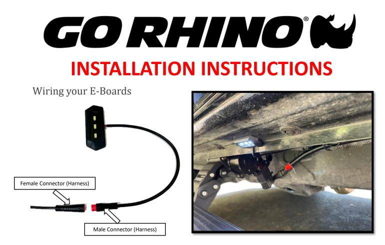
**Step 11**: Align the arrows on the small round connectors and plug the Passenger side front and Passenger side rear LED lights. Prepare the surface by cleaning with a 50/50 mix of isopropyl alcohol and water or equivalent. Once the surface is completely dry, peel the backing from the double-sided tape and stick the LEDs to the bottom side of the rocker panel. Position the LED lights at the center of the front and rear passenger side doors
