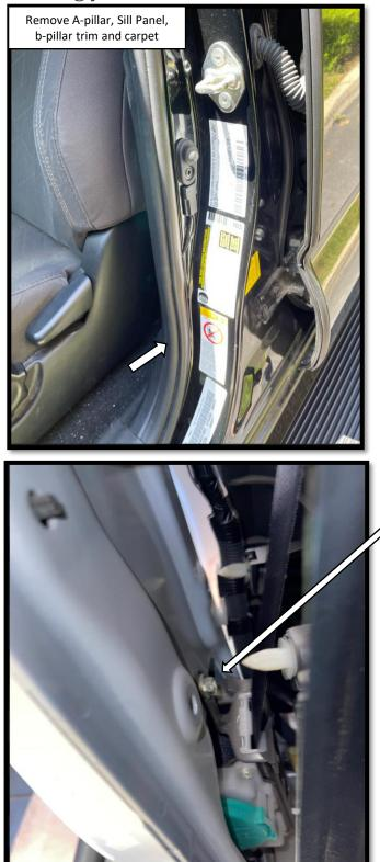
**Step 15:** Route the Driver side door trigger wire (brown) towards the Driver side b-pillar. Route the Passenger side door trigger wire (white) and the black disable switch wires under the center console to the left side of the vehicle. The white wire needs to go to the passenger side b-pillar, the black wires will go to the center console.
