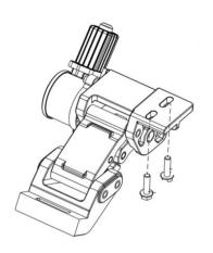
**Step 4**: Install the Front DRIVER side motor using (2) M8X30mm Flange Bolts, to fasten the motor to the vehicle. The hardware should be hand tightened only until snug. This will allow the motor assembly to move and align easier when installing the running board.
