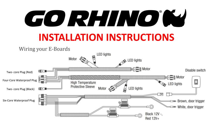
**Step 9:** Route the electrical harness from the controller along the frame rail of the vehicle. Connect the male plug connector on the wire harness into the female socket on the motors. The harness is labeled to show where to plug each male connector to the female connector. For example, Front Left is for the front Driver side motor and Rear Left for the rear Driver side motor. Use supplied zipties to secure harness to the frame rail.
