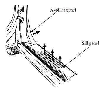
**Step 13:** On the DRIVER side, remove the front kick panel, front door sill trim panel and b-pillar trim panel. Go under the passenger seat and locate the split in the carpet. Pull the rear half of the carpet back to expose the oval rubber drain plug. Pull the drain plug and drill a 7/16" hole.
