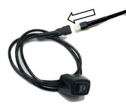
**Step 22:** Locate the black wires for the disable switch and feed them to your desired mount location. Prepare the surface by cleaning with a 50/50 mix of isopropyl alcohol and water or equivalent. Once the surface is dry, peel the backing from the double-sided tape and stick the disable switch on the lower dash panel. Plug the disable switch connector into the black wire harness and tuck the extra wire behind the lower dash panel.
