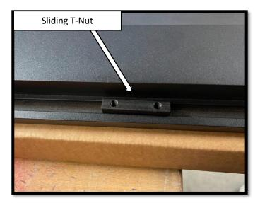
**Step 7**: Install the Driver side running board. With assistance, begin by positioning the board on the front and rear motor assembly bases. Align the sliding T-Nut on the running board with the slots on the front and rear motor base. Once the T-Nuts are aligned, rotate the running board so that the T-Nuts set in the slots on the base of the arms. Repeat 1-6 to install the motor linkage assemblies and running board on the Passenger side side.
