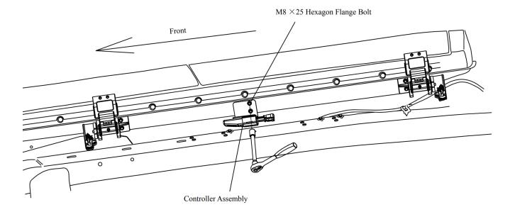
**Step 6**: Install the CONTROL MODULE on DRIVER side center mount side motor using (2) M8X25mm Flange Bolts.
