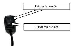
**Step 24:** Open the Driver side door and keep the door open. Flip the disable switch to the Off position. This will signal the running boards to retract to the stowed position and it will disable any further operation until the switch is flipped to the On position.
