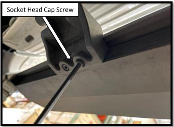
**Step 7**: Determine where you want to position the board and secure the running board to the arms using the (2 per bracket) M6x25 socket head cap screws. Using a torque wrench, tighten to 9 ft-lbs. Step # With the running board is installed, fasten the hardware on the driver side front and rear motor assemblies. Using a torque wrench, tighten the mounting hardware to 18 ft-lbs.
