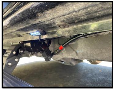
**Step 11**: Align the arrows on the small round connectors and plug the Driver side front and Driver side rear LED lights. Prepare the surface by cleaning with a 50/50 mix of isopropyl alcohol and water or equivalent. Once the surface is completely dry, peel the backing from the double-sided tape and stick the LEDs to the bottom side of the rocker panel. Position the LED lights at the center of the front and rear passenger side doors
