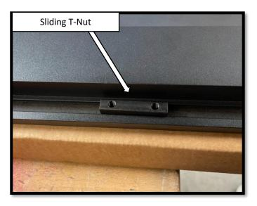
**Step 6**: Install the DRIVER side running board. With assistance, begin by positioning the board on the front and rear motor assembly bases. Align the sliding T-Nut on the running board with the slots on the front and rear motor base. Once the T-Nuts are aligned, rotate the running board so that the T-Nuts set in the slots on the base of the arms. Repeat 1-14 to install the motor linkage assemblies and running board on the PASSENGER side side.
