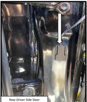
**Step 19: REAR DOOR** Apply a vertically oriented strip of masking tape on the rear Driver side door using the door stopper as a reference point. Make a mark 3.5" below the center line of the latch. Prepare the surface by cleaning with a 50/50 mix of isopropyl alcohol and water or equivalent. Once the surface is completely dry, peel the backing from the double-sided tape and stick the magnet to the door. Align the top of the magnet with the 3.5" mark as shown.
