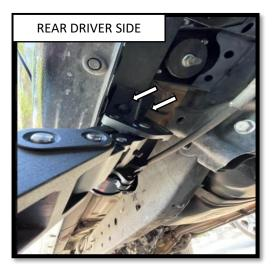
**Step 3**: Install the REAR DRIVER side motor using (2) M8X30mm Flange Bolts, to fasten the motor to the vehicle. The hardware should be hand tightened only until snug. This will allow the motor assembly to move and align easier when installing the running board.
