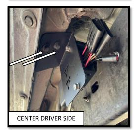
**Step 5**: Install the CONTROL MODULE on driver side center mount side motor using (2) M8X25mm Flange Bolts.
