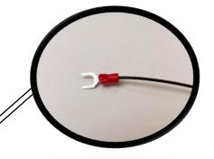
**Step 16:** The door trigger sensor harness will need a ground connection to the vehicle. Locate the seat belt assembly at the passenger side b-pillar and install the ground wire under the top bolt of the seat belt assembly.
