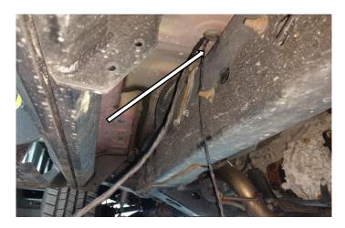
**Step 14:** Go under the vehicle and feed the door trigger signal wires (white and brown) and the disable switch wires (two black wires) into the cab. Feed the wires thru the hole in the rubber drain plug. Pop the drain plug back into the slot. Seal around the wires using RTV silicone adhesive to prevent water intrusion. These cables will run underneath the driver side seat.
