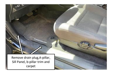
**Step 13:** On the DRIVER side, remove the front kick panel, front door sill trim panel and b-pillar trim panel. Go under the passenger seat and locate the split in the carpet. Pull the rear half of the carpet back to expose the oval rubber drain plug. Pull the drain plug and drill a 7/16" hole.
