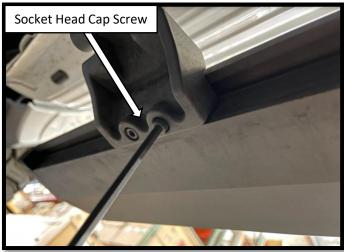
**Step 7**: Determine where you want to position the board and secure the running board to the arms using the (2 per bracket) M6x25 socket head cap screws. Using a torque wrench, tighten to 9 ftlbs. Step # With the running board is installed, fasten the hardware on the Passenger side front and rear motor assemblies. Using a torque wrench, tighten the mounting hardware to 18 ftlbs.
