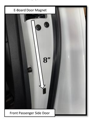
Step 17: FRONT DOOR Apply a vertically oriented strip of masking tape on the front Passenger side door using the deepest part of the latch as a reference point. Make a mark 8" below the center line of the latch. Prepare the surface by cleaning with a 50/50 mix of isopropyl alcohol and water or equivalent. Once the surface is completely dry, peel the backing from the double-sided tape and stick the magnet to the door. Align the top of the magnet with the 8" mark as shown.
