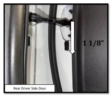
Step 19: REAR DOOR Apply a vertically oriented strip of masking tape on the rear Driver side door using the door stopper as a reference point. Make a mark 1 1/8" below the center line of the latch. Prepare the surface by cleaning with a 50/50 mix of isopropyl alcohol and water or equivalent. Once the surface is completely dry, peel the backing from the double-sided tape and stick the magnet to the door. Align the top of the magnet with the 1 1/8" mark as shown.
