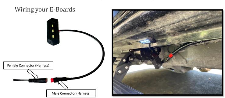
**Step 11**: Align the arrows on the small round connectors and plug the Passenger side front and Passenger side rear LED lights. Prepare the surface by cleaning with a 50/50 mix of isopropyl alcohol and water or equivalent. Once the surface is completely dry, peel the backing from the double-sided tape and stick the LEDs to the bottom side of the rocker panel. Position the LED lights at the center of the front and rear passenger side doors
