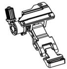
**Step 3**: Install the Front passenger side motor using (3) M8X30mm Flange Bolts, to fasten the motor to the vehicle. The hardware should be hand tightened only until snug. This will allow the motor assembly to move and align easier when installing the running board.
