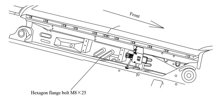
**Step 6**: Install the CONTROL MODULE on Passenger side center mount side motor using (2) M8X25mm Flange Bolts.
