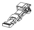
**Step 4**: Install the Center Idler Bracket on passenger side using (2) M8X30mm Flange Bolts, to fasten the motor to the vehicle. The hardware should be hand tightened only until snug. This will allow the motor assembly to move and align easier when installing the running board.
