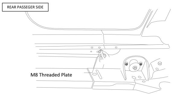
Step 3: : Install the rear passenger side motor mounting bracket using an M8 stud bolt
