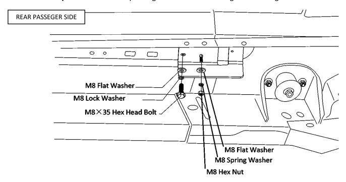
**Step 4**: Install the rear passenger side motor mounting plate using M8x35 Hex Bolt (1), M8 Lock Washer (1), M8 Flat Washer (1) on the exposed threaded hole. On the M8 Threaded Stud, fasten it with m8 Hex Nut (1), M8 Lock Washer (1), M8 Flat Washer (1). Torque down to 17 FT LBS.
