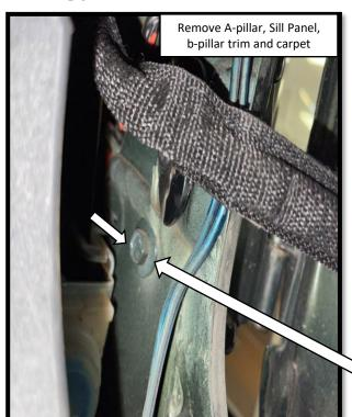
**Step 20:** Route the passenger side door trigger wire (brown) towards the passenger side b-pillar. Route the driver side door trigger wire (white) and the black disable switch wires under the center console to the left side of the vehicle. The white wire needs to go to the driver side b-pillar, the black wires will go to the center console.
