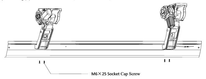
**Step 8**: Install the Passenger side running board. With assistance, begin by positioning the board on the front and rear motor assembly bases. Align the sliding T-Nut on the running board with the slots on the front and rear motor base. Once the T-Nuts are aligned, rotate the running board so that the T-Nuts set in the slots on the base of the arms. Repeat **1-11** to install the motor linkage assemblies and running board on the driver side side.
