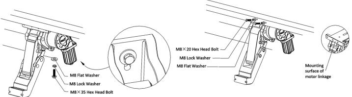
**Step 6**: Install front passenger side bracket onto weld seam using (2) M8x20MM Hex Bolts, M8 Lock Washer, M8 Flat Washer. On the underside of the bracket, secure it to the motor to the mounting plate using (1) M8x35MM Hex Bolts, M8 Lock Washer, M8 Flat Washer.
