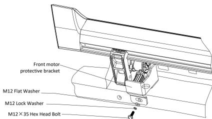
**Step 11**: Install the passenger side front motor protective bracket. Secure the protective bracket using an M12 hex bolt, flat washer, and lock washer. Torque to 25 ft-lbs.
