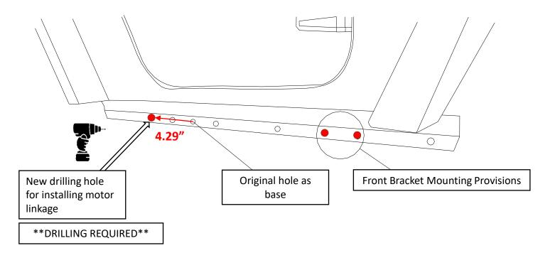
**Step 5**: . Using a measuring tape, measure 4.29"from the forward mounting hole. Use a center punch to mark the hole location and drill the 21/64" hole. Use touch up paint to cover up any raw metal on the pinch seam. You can check to see if you placed the hole in the correct location by mocking the bracket up against the weld seam. Using a 21/64" drill bit, chase the two front motor mounting holes on the pinch seam. Use touch up paint to cover up any raw metal on the pinch seam.
