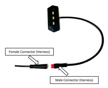
**Step 16**: Align the arrows on the small round connectors and plug the Passenger side front and Passenger side rear LED lights. Prepare the surface by cleaning with a 50/50 mix of isopropyl alcohol and water or equivalent. Once the surface is completely dry, peel the backing from the double-sided tape and stick the LEDs to the bottom side of the rocker panel. Position the LED lights at the center of the front and rear passenger side doors
