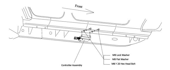
**Step 12**: Find the middle two holes on the pinch seam below the passenger side door. Using two M8 hex head bolts, M8 flat washers and M8 lock washers, install the controller mounting bracket. Using a torque wrench, tighten to 18 ft-lb.
