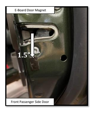
Step 22: FRONT DOOR Install front magnet (small) onto the front passenger side door about 1.5" below the center line of the latch. Prepare the surface by cleaning with a 50/50 mix of isopropyl alcohol and water or equivalent. Once the surface is completely dry, peel the backing from the double-sided tape and stick the magnet to the door. Align the top of the magnet with the 1.5" mark as shown. Verify that the magnet should be in line with the door sensor.
