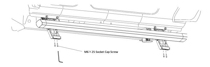
**Step 10**: Install the Passenger side running board. With assistance, begin by positioning the board on the front and rear motor assembly bases. Align the sliding T-Nut on the running board with the slots on the front and rear motor base. Once the T-Nuts are aligned, rotate the running board so that the T-Nuts set in the slots on the base of the arms. Repeat 1-14 to install the motor linkage assemblies and running board on the driver side side.
