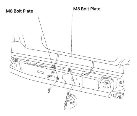
**Step 8**: Locate the paired square holes in the center of the body and insert the M8 bolt plates inside.
