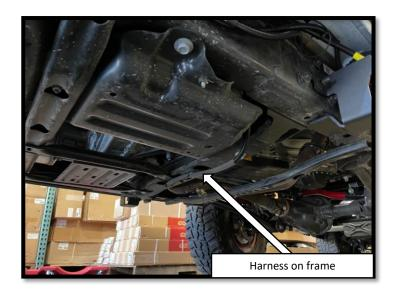
**Step 16**: Route the motor and LED wire harness from the controller to the Passenger side frame rail of the vehicle. When routing the harness keep clear from any moving parts and avoid direct contact with the exhaust system.
