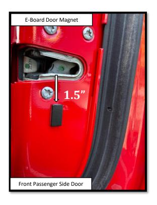
Step 21: FRONT DOOR Apply a vertically oriented strip of masking tape on the front Passenger side door using the deepest part of the latch as a reference point. Make a mark 1.5" below the center line of the latch. Prepare the surface by cleaning with a 50/50 mix of isopropyl alcohol and water or equivalent. Once the surface is completely dry, peel the backing from the double-sided tape and stick the magnet to the door. Align the top of the magnet with the 1.5" mark as shown.
