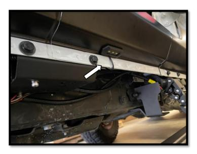
**Step 15**: Align the arrows on the small round connectors and plug the Passenger side front and Passenger side rear LED lights. Prepare the surface by cleaning with a 50/50 mix of isopropyl alcohol and water or equivalent. Once the surface is completely dry, peel the backing from the double-sided tape and stick the LEDs to the bottom side of the rocker panel. Position the LED lights at the center of the front and rear passenger side doors
