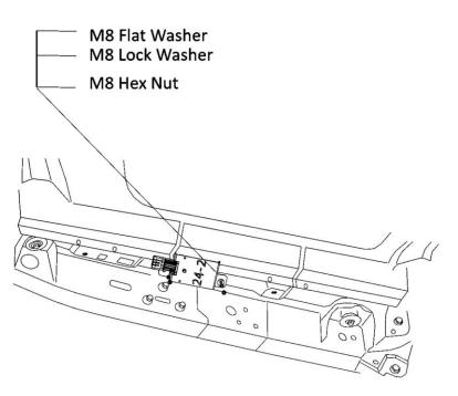
**Step 9**: Using two M8 hex head bolts, M8 flat washers and M8 lock washers, install the controller mounting bracket. Using a torque wrench, tighten to 18 ft-lb
