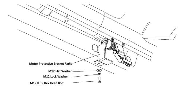
**Step 7**: Install the passenger side front motor protective bracket. Secure the protective bracket using an M12 hex bolt, flat washer, and lock washer. Torque to 25 ft-lbs.
