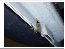
Insert a U-bolt into the top two drilled holes as shown.
