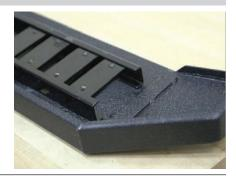
Carefully place the running board onto the mounting brackets.
