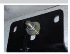
Moving to the passenger side of the vehicle, identify the front bracket location by identifying the slot in the rocker panel.
