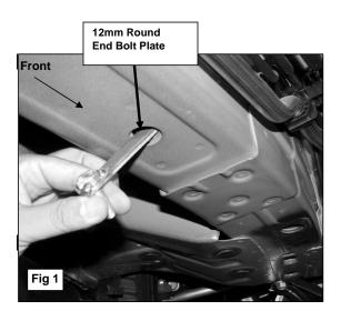
8mm x 25mm Hex Bolts 8mm x Flat Washers 12mm Round End Bolt Plate (Rotate Bolt Plates 90-degrees after installing)
