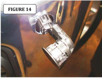
**Step-9** Remove the sensor plates that are preinstalled in the BR6 bumper. Discard the plastic plugs from the sensor plates.
