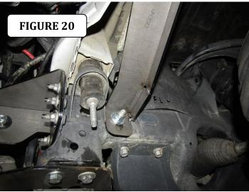
**Step-14** Secure the driver side support bracket to the frame using the T-Bolt, (1)  $\frac{1}{2}$ " flat washer, (1)  $\frac{1}{2}$ " lock washer and (1)  $\frac{1}{2}$ " hex nut, (FIGURE 20). Attach the opposite end of the support bracket to the bumper shell bracket using (1)  $\frac{3}{8}$ " x 1  $\frac{1}{4}$ " hex bolt, (1)  $\frac{3}{8}$ " lock washer, (2)  $\frac{3}{8}$ " flat washers and (1)  $\frac{3}{8}$ " hex nut, (FIGURE 21). Leave the bolts loose for final adjustment.
