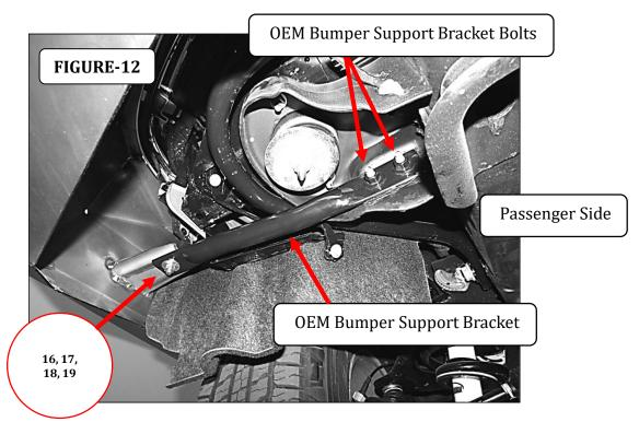
**Step-9** With assistance, adjust and hold the bumper shell visual alignment position, then tighten all factory and supplied nuts and bolts securing the brackets, winch tray and bumper shell.
