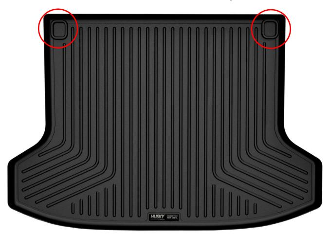
YOUR CARGO LINER HAS ACCOMMODATIONS TO ALLOW ACCESSING THE FACTORY CARGO TIEDOWN HOOKS WITH THE LINER INSTALLED. TO ACCESS THE HOOKS SIMPLY TRIM AWAY THE MATERIAL FROM ANY OR ALL OF THE TIE-DOWN LOCATIONS (SHOWN ABOVE CIRCLED). TO AID IN TRIMMING THE AREAS ARE RECESSED IN THE PART. A UTILITY KNIFE WORKS WELL FOR TRIMMING.
