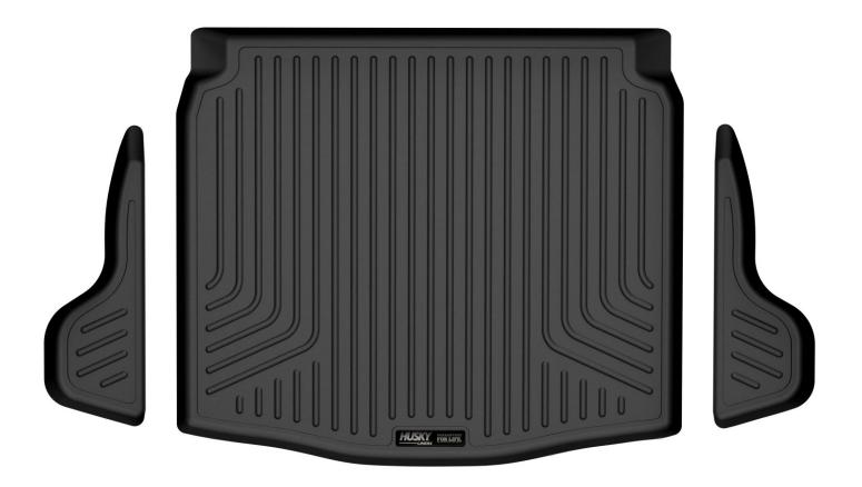
THE TWO SMALLER LINERS WILL FIT INTO THE TWO LOWER-LEVEL AREAS LOCATED BEHIND EACH WHEEL WELL OF THE VEHICLE. CERTAIN VEHICLE TRIM LEVELS WILL ONLY HAVE ONE LOWER LEVEL AREA.
