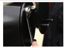
Lift the spare tire back onto the three mounting lugs and secure with the factory lug nuts.
