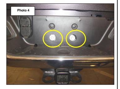
**Step-6** Remove the bolts (2) per side securing the factory bumper brackets to the frame/receiver hitch using a 15mm socket and ratchet, (Photo 5).
