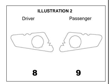
**Step-5** Prepare the inside of the replacement bumper surface where the bezel plates will be mounted with Isopropyl alcohol. A clean, dry surface is required in order for tape to stick properly.
