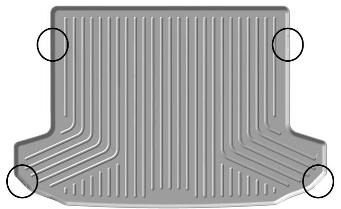
YOUR TUCSON HAS FOUR (4) CARGO TIE DOWN HOOKS LOCATED AROUND THE PERIMTER OF THE CARGO AREA. TO ACCESS TO THE FACTORY TIE-DOWN HOOK LOCATIONS (SHOWN CIRCLED ABOVE) WITH THE LINER IN PLACE. SIMPLY REMOVE/TRIM THE MATERIAL FROM THE PORTION OF THE LINER OVERLAPPING THE HOOKS. THESE AREAS ARE RECESSED ON THE LINER TO GUIDE TRIMMING. A UTILITY KNIFE WORKS WELL FOR TRIMMING.
