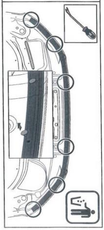
Gently peel back the rubber seal and insert a screw plug into the vacant holes in the underside of the hood.
