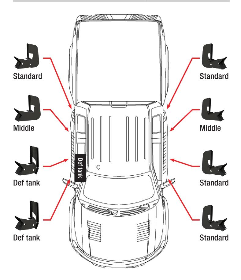
Starting on the driver side, locate the five mounting locations underneath the vehicle.
