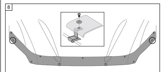
**7•** Slide the two metal Push-on clips over the abrasive resistant tape on the hood edge at the two previously noted outer positions.
