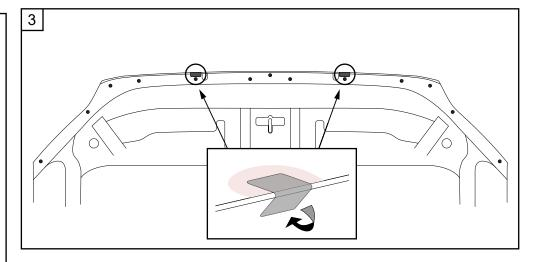
4. Install the two Fixed Clips by aligning them with the previously noted holes in the hood. Insert the Screw Plugs through the rectangular holes of the Fixed Clips into the hood. While pushing the Screw Plug down against the Fixed Clip insert the two self-tapping screws into the Screw Plugs.
