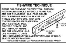
6. Reverse fishwire 1/2-13 x 1 3/4" carriage bolts and SP6 spacers into the access holes.
