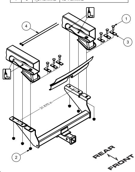
1. Determine if trimming is required on model by raising hitch into position. If needed, mark and trim lower fascia or remove lower fascia and return to owner. (See fascia trim detail) **Note:** Check for proper fit prior to trimming.
