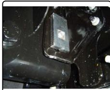
4. Raise hitch into position and push bolts out. Attach M12-1.75 hex flange nut to bottom bolt on each side. Re-attach (2) nuts removed in STEP 2 to top bolt on each side.
