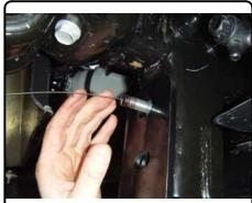
6. Torque all M12 hardware to 79 ft-lbs and 7/16 in hardware to 70 ft-lbs.
