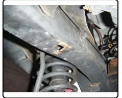
Fishwire (2) carriage bolts and (2) CM-SP6 spacers into position in the side of each frame rail. Reverse fishwire (1) carriage bolt and (1) CM-SP6 spacer into position in the bottom of each frame rail. NOTE: Leave fishwires attached to all hardware to prevent hardware becoming lost in frame.
