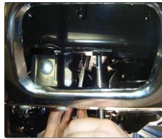
6. Assemble center hitch to side plates using 7/16" hardware as shown in <u>ILLUSTRATION</u> and pictures below.
