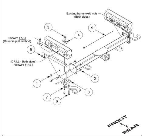
1. Remove tow hooks and set aside for later reattachment. Hardware to be returned to vehicle owner and will not be reused.
