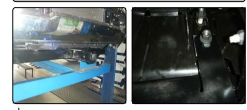
4. Rotate the hitch against the frame rails. Mark the bottom holes for drilling. If a hole exists on the side of the frame rail near the hitch, enlarge the hole to allow the carriage bolts and CM-SP40 spacers to pass through. Drill the bottom of the frame rails for 1/2" hardware. If no hole exists, remove the hitch and use the hole saw to drill a hole in the bottom of the frame rails.
