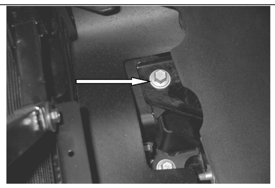
**STEP 1.** BEGINNING WITH THE PASSENGER SIDE, LOCATE AND REMOVE THE UPPER BUMPER BOLT. THE BOLT IS LOCATED BEHIND THE GRILLE ON THE TOP OF THE BUMPER. THE BOLT IS ACCESSIBLE BY REMOVING THE RIVETS AND PLASTIC TRIM PANEL ON TOP OF THE GRILLE, AND REACHING DOWN THROUGH THE OPENING.
