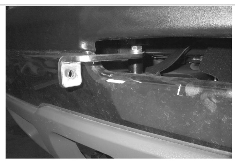
STEP 2. POSITION 1100AP UPPER BRACKET THROUGH THE OPENING IN THE BUMPER. LOOSELY ATTACH THE BRACKET TO THE BUMPER USING THE 12MM X 70MM BOLT, TUBULAR SPACER AND ½" WASHERS.
