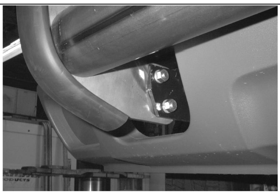
**STEP 7.** ATTACH THE GRILLE GUARD ASSEMBLY TO THE OUTSIDE OF THE FRAME BRACKETS, AND UPPER BRACKETS USING THE 3/8" X 1" BOLTS, LOCK WASHERS, AND NUTS. ALIGN THE GRILLE GUARD ASSEMBLY WITH THE FRONT OF THE VEHICLE AND TIGHTEN ALL NUTS AND BOLTS.
