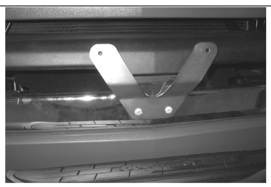
**STEP 6.** REMOVE THE LICENSE PLATE AND MOUNTING BRACKET FROM THE FRONT BUMPER. ATTACH 1100LP LICENSE PLATE BRACKET TO THE BUMPER USING THE FACTORY SCREWS, AND THE LICENSE PLATE TO THE BRACKET USING THE 1/4" FASTENERS SUPPLIED.
