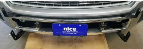
With the brackets installed, lift the guard (with assistance) into place and install one M8 x 30mm hex bolt, two M8 flat washers and one M8 nylock nut into the top bracket.
