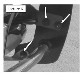
**Step-6** Attach the side plates to the lower brackets using (1) 1/2" X 1 1/2" hex bolts, (1) 1/2" flat and lock washers and (1) 1/2" hex nut by each side. Do not tighten. Picture 6.
