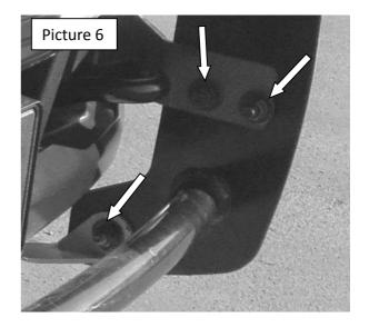
**Step-6** Attach the side plates to the lower brackets using (1)  $1/2^{"} \times 1 1/2^{"}$  hex bolts, (1)  $\frac{1}{2}^{"}$  flat and lock washers and (1)  $\frac{1}{2}^{"}$  hex nut by each side. Do not tighten. Picture 6.
