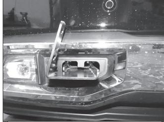
(Fig 11) Passenger/right side Bracket installed
