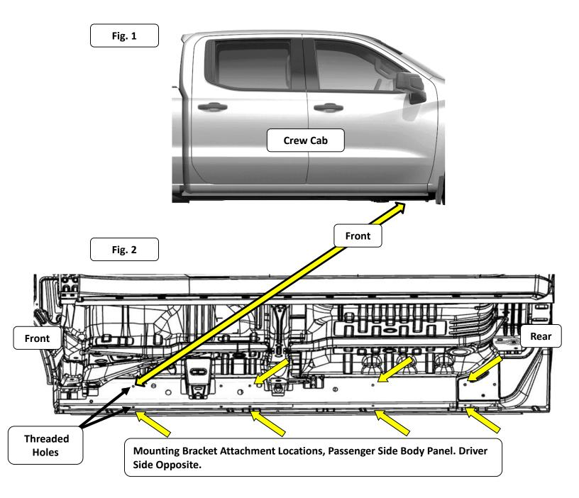
**Step-2** Attach one of the brackets to the body panel using (2) M8 X 25mm hex bolts, (2) 5/16" lock washers and (2) 5/16" flat washers, (Fig. 3). Do not tighten the bolts.
