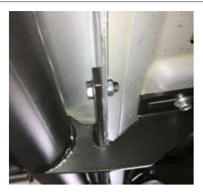
**Step 6.** Continue installing the rest of the hardware in the front brackets and leave loose.
