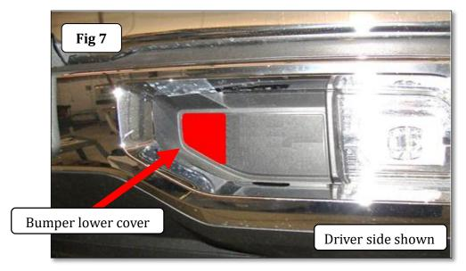
**Step-2b** From behind the bumper position the driver side mounting bracket [Item M] through the opening cut out in the bumper lower cover and up to the side of the frame.
