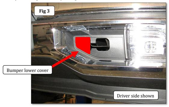
**Step-4a** From behind the bumper position the driver side mounting bracket through the opening in the bumper lower cover and up to the side of the frame. Align the (2) holes in the mounting bracket with the holes in the frame, and re-install the tow hook and tow hook bolts and nut to secure the mounting bracket and tow hook, (Fig 4). Snug but do not tighten the bolts and nut.
