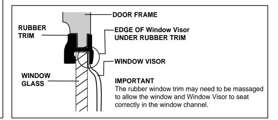
IMPORTANT: Before fitting product, read instruction fully. Full tape strength is achieved after 72hrs. Allow tape to cure for 4hrs before driving vehicle. Reverse the above procedure to remove this product.
