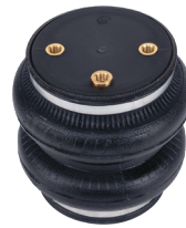
LoadLifter 5000 Zytel ® plastic end cap
