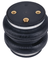
LoadLifter 5000 Ultimate Zytel® plastic end cap
