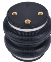
Air Lift® ProSeries (77-Series) Zytel® plastic end cap
