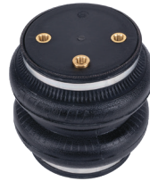
LoadLifter 5000 Zytel® plastic end cap
