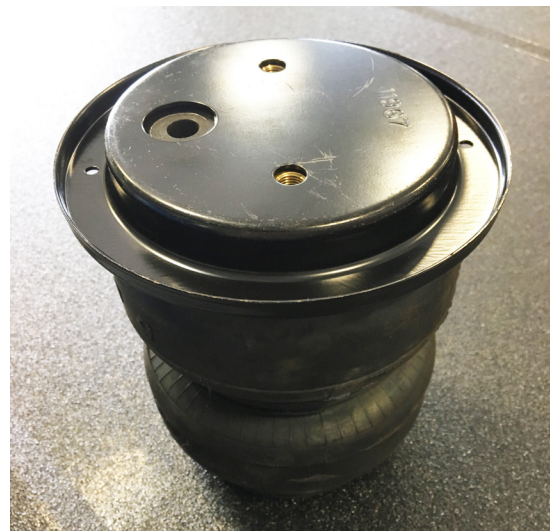
If no spacer needed (roll plate only) use the included shorter hardware
