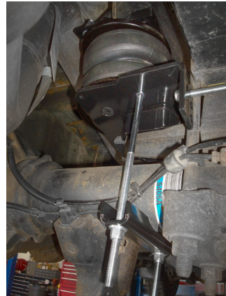
Back passenger's side (right) rear view of the kit installed.
