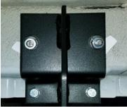
Using the 3" U-Bolt put it through the top 2 mounting holes and secure with (2) plastic bolt retainer.
