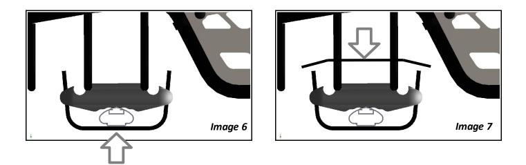
**6.** Secure each thread of the "U"-bolt with a Knob nut.
