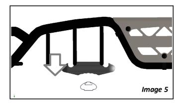
**5.** Place the (x4) fixation plates above the cross tubes, align them with each plastic holder, then place the (x4)"U"-bolts below the roof bars.
