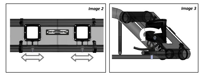
**3.** Install safari rack. Place the (x4) plastic holders below the safari rack and close to the edges. Distribute them at the same distance from center then snap them between the cross tubes.
