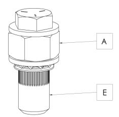
Hand tighten <sup>1</sup>/<sub>4</sub>" rivet nut onto installation tool • as shown.
