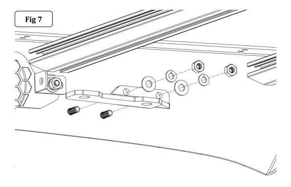
**Step-8** Repeat Step 5, 6 and 7 to attach the brackets to the side rail on driver side.
