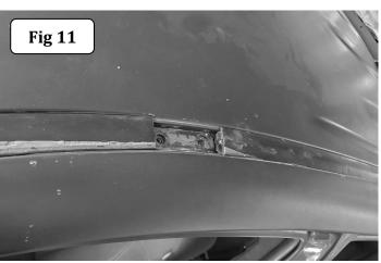
**Step-11** Cut the roof molding trim at marked areas. Install back the top molding trim and place the spacers over the holes (Fig 11).
