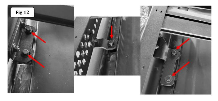
**Step-10** Adjust and align the SRM300 roof rack assembly as necessary and fully tighten all hardware.
