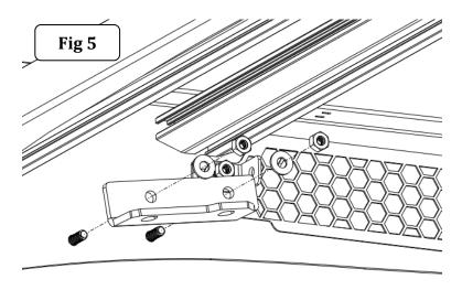
**Step-6** Install (1)  $\frac{1}{4}$ " x 1" button head screws with  $\frac{1}{4}$ " plastic washer in the central hole of the side rail. Place the center bracket onto the side rail, align the screws with the hole in the center bracket. Secure the center bracket using (1)  $\frac{1}{4}$ " lock washer, (1)  $\frac{1}{4}$ " flat washer and (1)  $\frac{1}{4}$ " hex nut. Snug but do not tighten the screw, (Fig 6).
