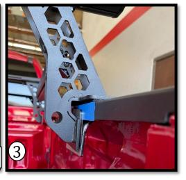
Use the provided bed rail clamp and install 5/16" carriage bolt from the backside (image 1). Place clamp spacer plate onto the bed rail clamp so that it acts as a spacer to square the clamp against the inside of the bed rail (image 2). Once the threads are exposed, position the clamp against the inside of the bed rail and use 5/16" flat washer, 5/16 lock washer, and 5/16 hex nut to secure the clamp. Leave finger tight for final adjustment. Repeat process for each corner.
