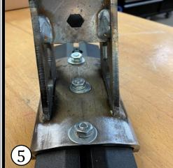
Install tower into crossbar with the  $\frac{1}{4}$ " exposed as studs (image 4). Secure each tower with 3 QTY with  $\frac{1}{4}$ " flat washer,  $\frac{1}{4}$ " lock washer,  $\frac{1}{4}$ " hex nut (image 5). Leave loose for final adjustment. Repeat steps for all four corners.
