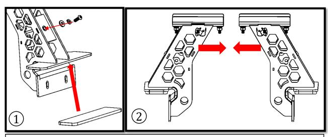
Install foam adhesive on the mounting surface of the SRM tower(image 1). Install  $\frac{1}{2}$ " button head screw,  $\frac{1}{2}$ " lock washer,  $\frac{1}{2}$ " flat washer onto the threaded riv-nut. Repeat steps for all four towers. Position each tower mounted be sure the Rhino heads are facing each other (image 2).
