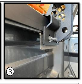
Use the provided bed rail clamp and install 5/16" carriage bolt from the backside (image 1). Place track system plate onto the bed rail clamp so that it acts as a spacer to square the clamp against the inside of the bed rail (image 2). Once the threads are exposed, position the clamp against the inside of the bed rail and use 5/16" flat washer, 5/16 lock washer, and 5/16 hex nut to secure the clamp. Leave finger tight for final adjustment. Repeat process for each corner.
