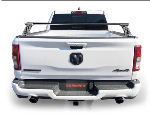
Once you position each tower and cross bar to your desired location, fasten all loose hardware. If bowing is present on the crossbars, loosen all hardware from the towers to the rail and make sure the cross bar is flat on the tower. Over tightening the tower onto the bed rail can result in cross bar bowing. Periodically inspect hardware and fasten as needed.
