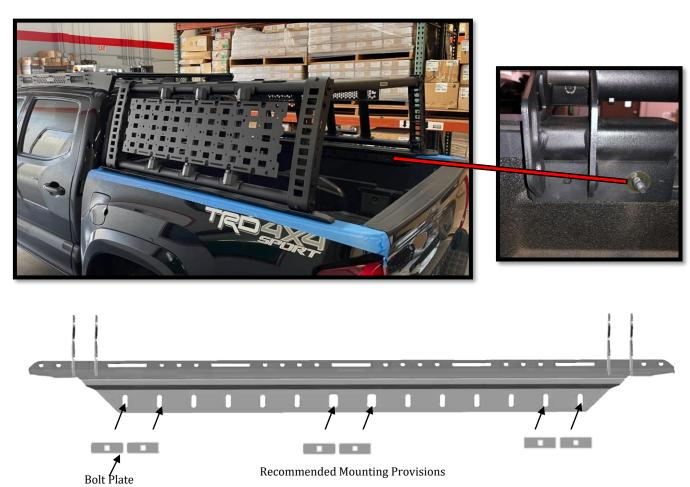
The feet on the XRS rack have a series of holes to allow for mounting in different locations. It is recommended to install the plates on the outer sides of the feet as well as in the center. This will help distribute clamping force
