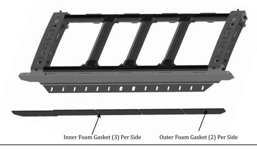
Before installing the XRS onto the truck bed, install supplied foam gaskets on the bottom surface of the rack feet. Each side will use (2) outer foam gaskets and (3) inner foam gaskets.
