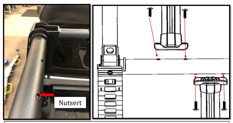
Install and seat each multi-core cross bar on the nutserts located on the connecting tubes. Long cross bars are installed on top, shorter cross bars are installed on the sides. Once installed, use  $\frac{1}{4}$ " x 3/4" button head SEMS bolt to secure cross bar to the connecting tube (2qty per side). Follow the same steps for the remaining multi-core cross bars and leave finger tight.
