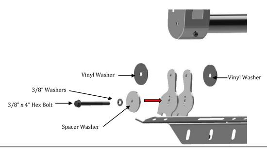
Install 3/8" x4" hex head bolt with 3/8" lock washer, 3/8 flat washer, Spacer Plate through the bottom hole of the upright. Before the bolt runs through, you will need to add (2) 2 ½' Vinyl Washer in between (one per side)
