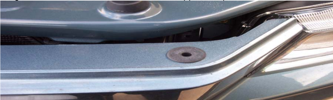
Diagram number 4. Trim panel re installed with Brace bracket installed
