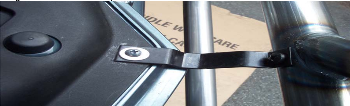
Diagram number 4. Trim panel re installed with Brace bracket installed
