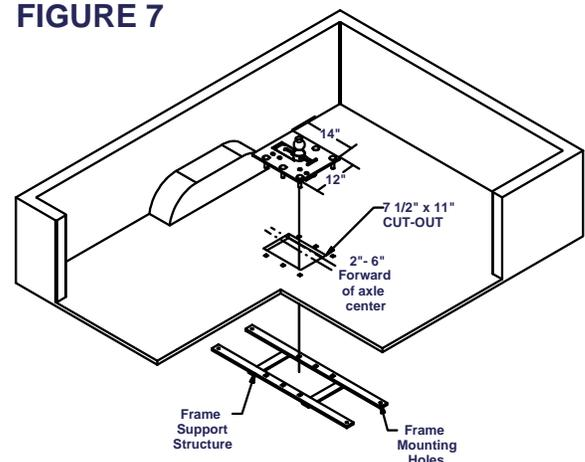
3. Place frame support structure underneath bed of truck and above truck frame. Align with cut-out in bed of truck. Use clamps to hold structure in place.
